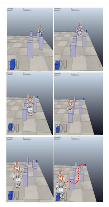
Fig. 1: Simulation result of NAO using PSO
